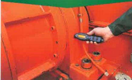
Checking the condition of bearings
